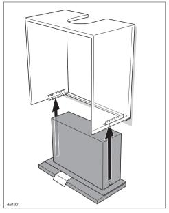
Insert the hood into the cabinet from below and until the spring clips click into place.
